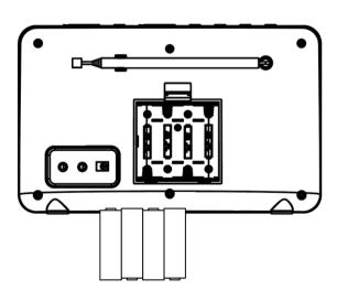
Note: For battery operation, please ensure that the mains power is switched off and remove the mains power plug from the socket, on the back of the Radio.
